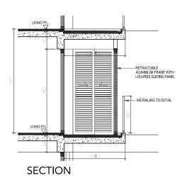
ALL BALCONIES SHALL NOT BE ENCLOSED UNLESS WITH THE APPROVED BALCONY SCREEN. FOR AN ILLUSTRATION OF THE APPROVED BALCONY SCREEN, PLEASE REFER TO THE ABOVE DIAGRAM. BALCONY SCREEN TO BE INSTALLED AT THE COST OF HOMEOWNERS.
